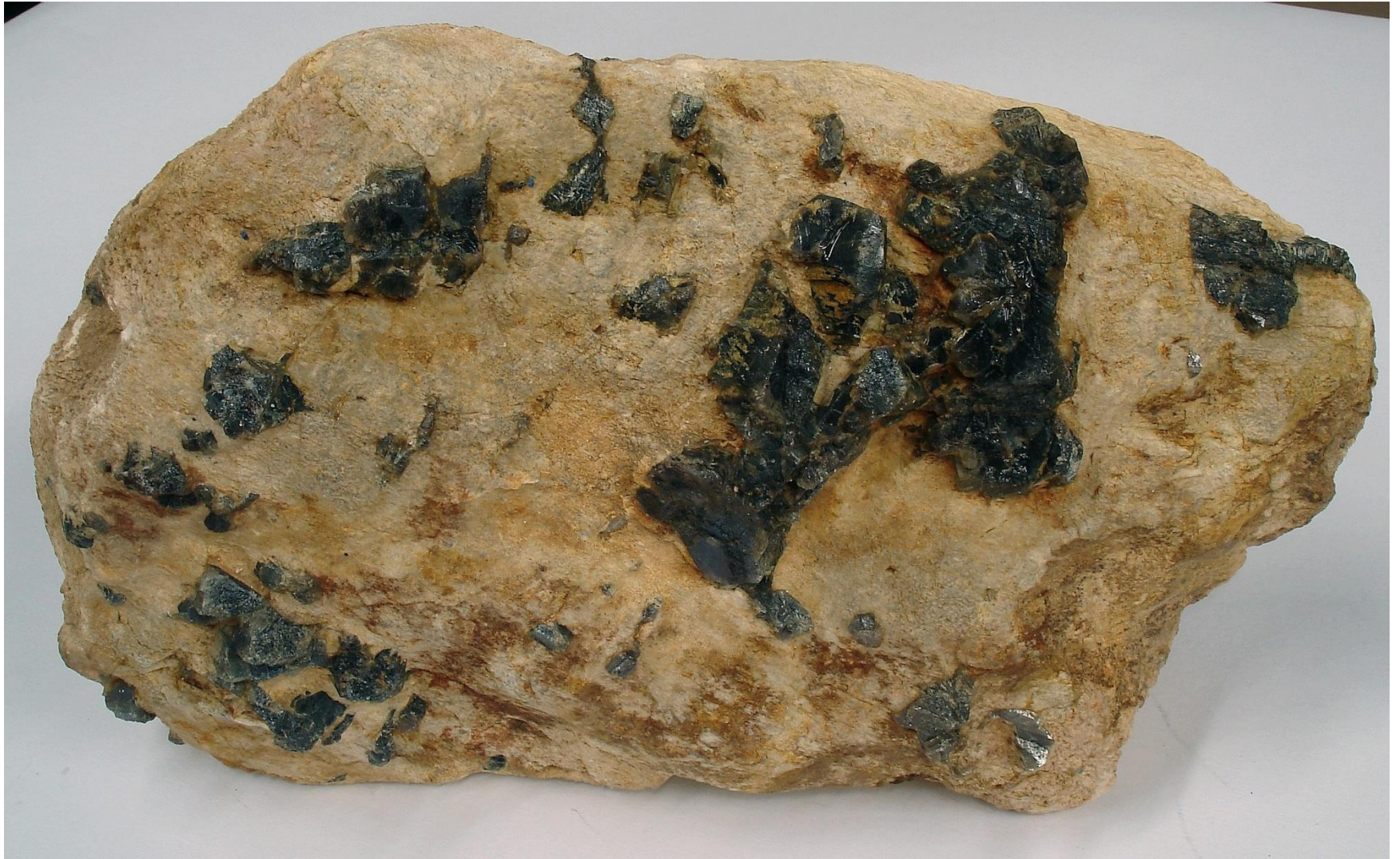
Sample of pegmatite composed mainly of altered feldspar, corundum and mafic minerals
